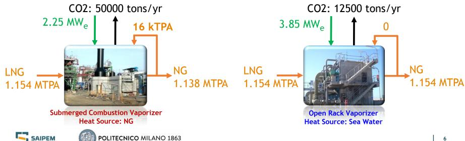
**TECHNOLOGY OVERVIEW Energy Recovery Performances** Performance indexes Target Specific Fuel Consumption (SCF) =  $\frac{Equivalent NG \ consumption}{regasified \ LNG} [kg_{NG}/tons_{LNG}]$  $\rightarrow 0$ Fuel Consumption Saving (FCS) =  $\frac{Consumption - SCV \text{ or } ORV \text{ consumption}}{SCV \text{ or } ORV \text{ consumption}} [\%]$  $\rightarrow$  -100
