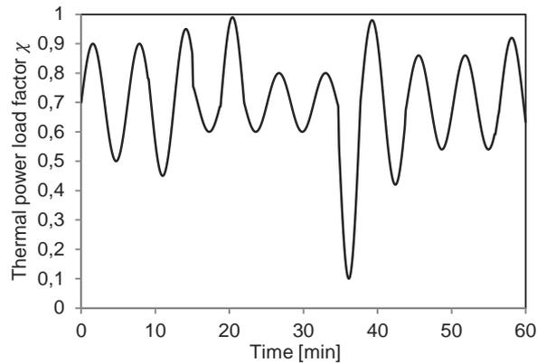
Fluctuating thermal power input means that the ORC system often experiences transients
