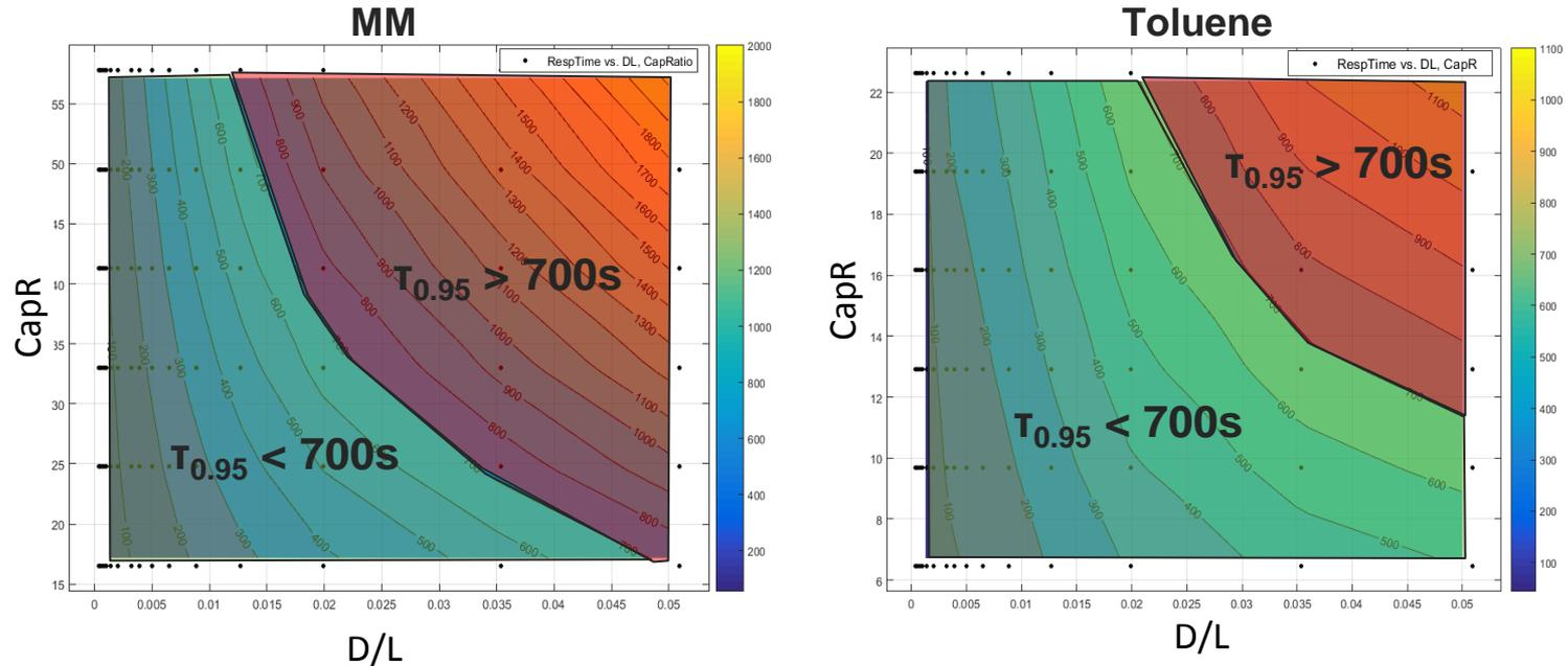
Comparison of resp times for two dif. Fluids with the same fixed parameters. (area, heat flux) → Toluene shows relatively shorter response times
