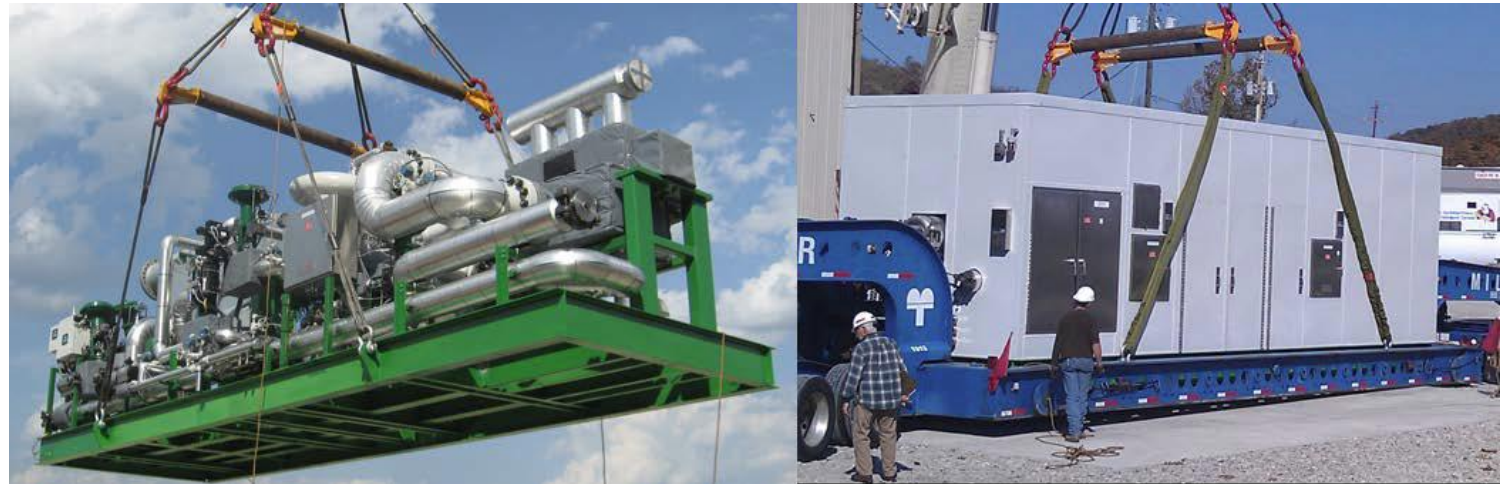
EPS100 sCO 2 heat engine, process and power skids (1)
