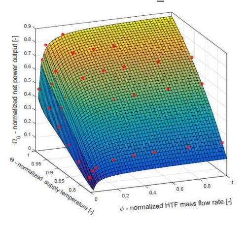
Effect of HTF mass flow rate  $\phi$ :
