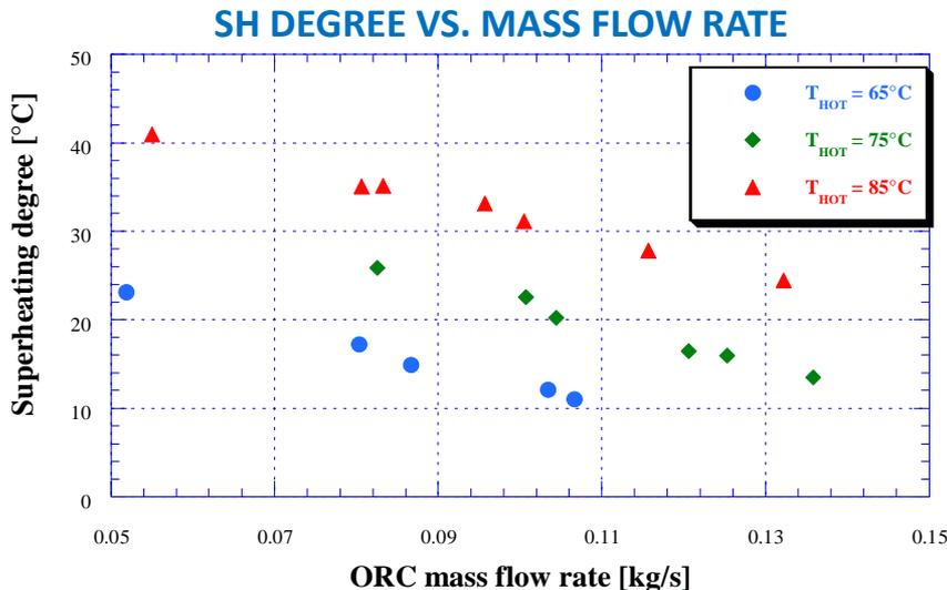
Superheating degree depending on mass flow rate and  $T_{HOT}$
