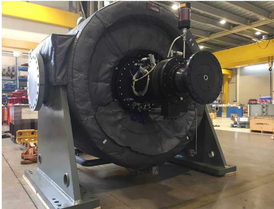
Five stage 16MW geothermal turbine adopting the new Turboden rotor design
