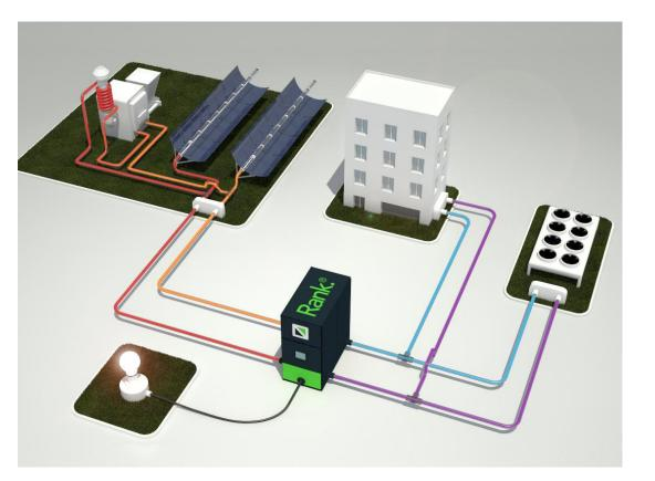
Combined Cold, Heat and Power (CCHP) using solar/biomass as renewable heat source
