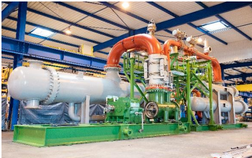
Organic Rankine Cycle (ORC) Generates electricity from heat
