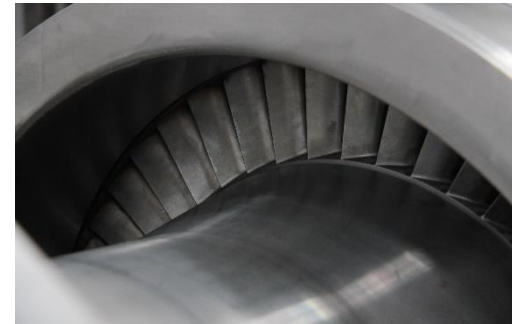
Natural gas Turbo-Expander Generates electricity by recovering energy from the gas expansion
